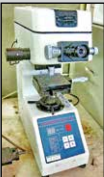
MICRO HARDNESS HV-1000 DIGITAL HARDNESS TESTER
