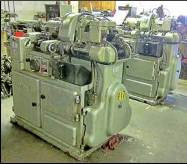
ESCOMATIC SINGLE-SPINDLE SCREW MACHINES
