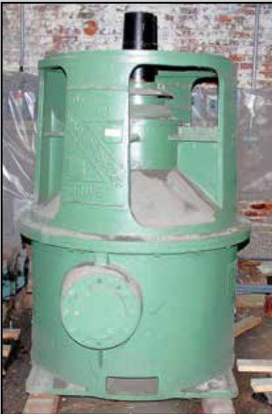
BLACK CLAWSON #3 HYDRAPULPER DRIVE, REBUILT
