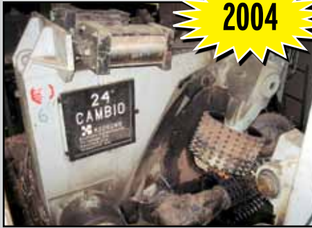
KOCKUMS CAMBIO 24" MECHANICAL RING DEBARKER
