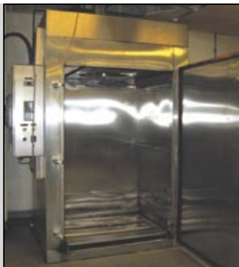
2000 KEMTEC STAINLESS STEEL RACK SMOKER, w/PLC CONTROLS
