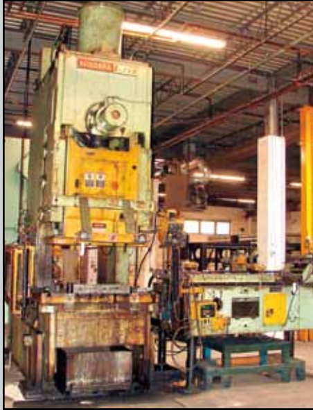
NIAGARA E-250 250-TON OBI PRESS AND COE 18" x 24" STRAIGHTENER
