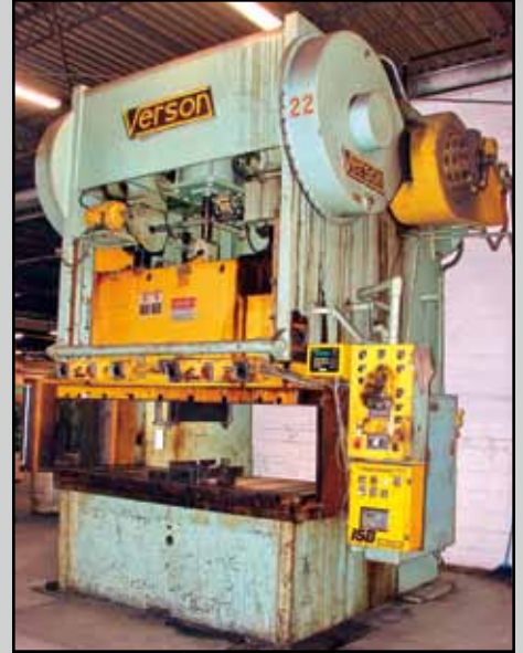
VERSON 300-TON STRAIGHT SIDE PRESS
