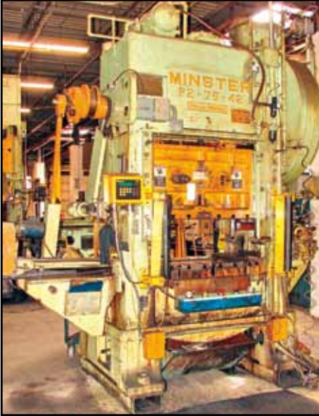
MINSTER PIECEMAKER 75-TON STRAIGHT SIDE PRESS
