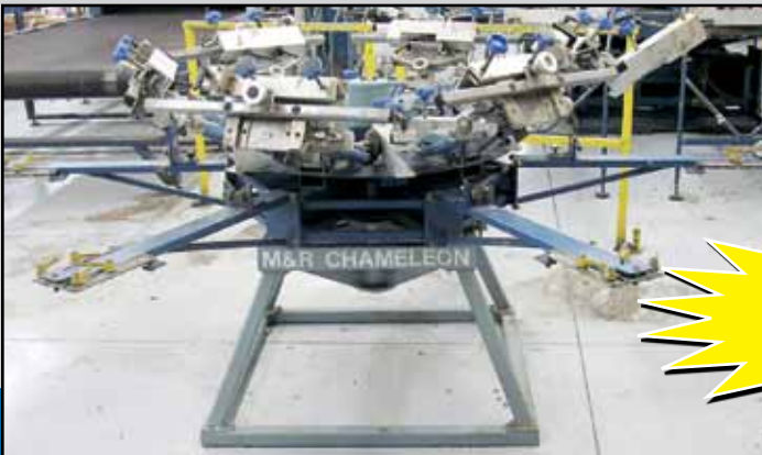
M&R CHAMELEON CHAM1-6-6 6 COLOR MANUAL ROTARY SCREEN PRESS
