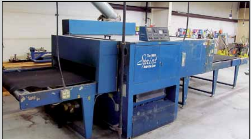
M&R TUNNEL DRYER
