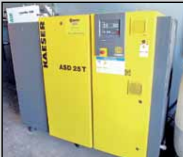
KAESER ASD25T 25 HP AIR COMPRESSOR
