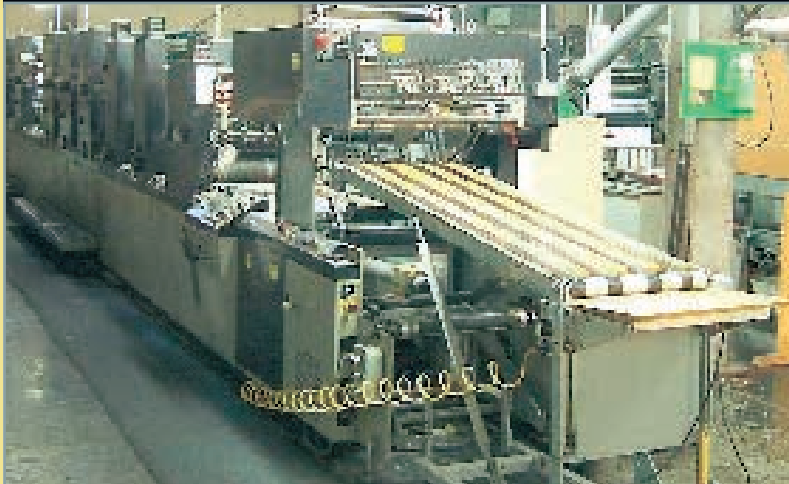
MAN-ASHTON Mdl. P-84 4-Color Continuous Form Printing Press, 20" x 22", w/roll feed, GWD web guide, numbering, perforation, punch, and slitting stations, Egan stacking unit, auto. registration, right-angle feed table, folder.
