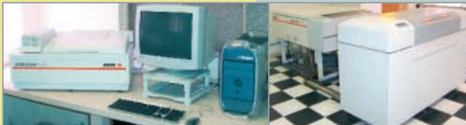
Electronic Pre-Press System , consisting of Agfa SelectSet 7000 image setter, Viper RIP w/Agfa Rapline 280LP image processor, Apple Macintosh G-3 computer system, Agfa Horizon Plus digital image scanner.
