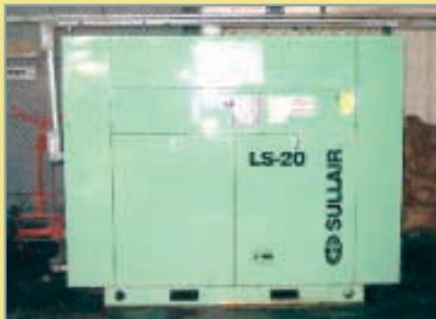
SULLAIR Mdl. LS20-100-ACAC 100 Hp. Rotary Screw Compressor , w/Pioneer refrigerated air dryer, vertical holding tank.
