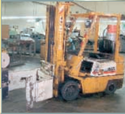
KOMATSU FG 18ST-2 3,000-Lb. Fork Truck, solid tire, LP, 185", 3-stage mast, side shift, hydraulic roll clamp attachment.
