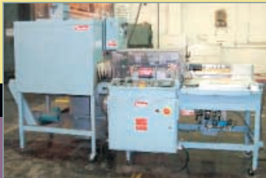
SHANKLIN A26A L-Bar Sealer, w/T7XL shrink wrap tunnel.
