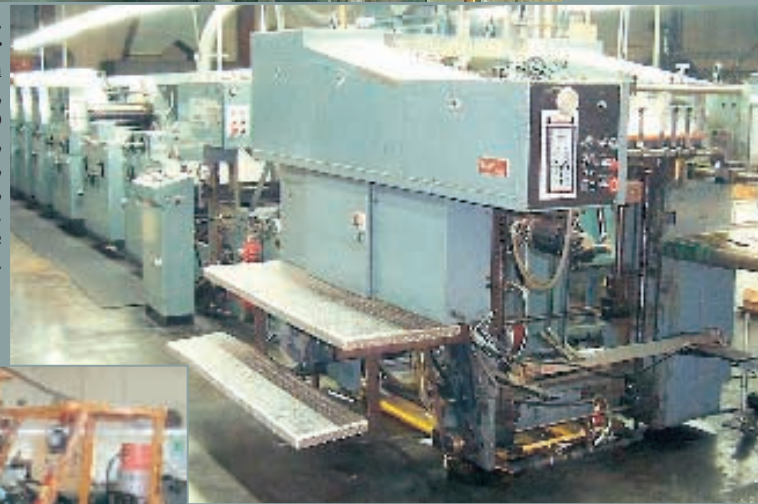
MAN-ASHTON Mdl. P-84 4-Color Continuous Form Printing Press, 20" x 22", w/roll feed, GWD web guide, numbering, perforation, punch, and slitting stations, Egan stacking unit, auto. registration, right-angle feed table, folder.
