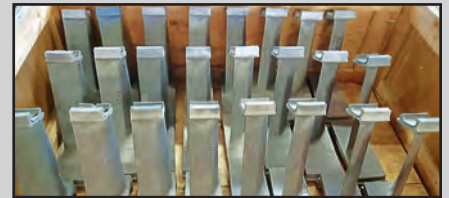
SIEMENS V84.2, ROW 3 VANES, P-N 02-8429-12-603 (PART OF COMPLETE SET)
