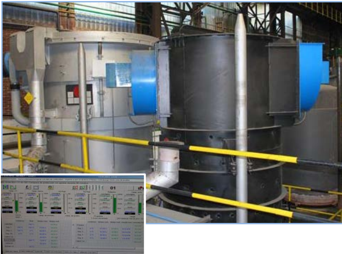
1500MM x 3700MM x 50TON LOI HYDROGEN 100%H2 BELL ANNEALING FURNACE, 2006
