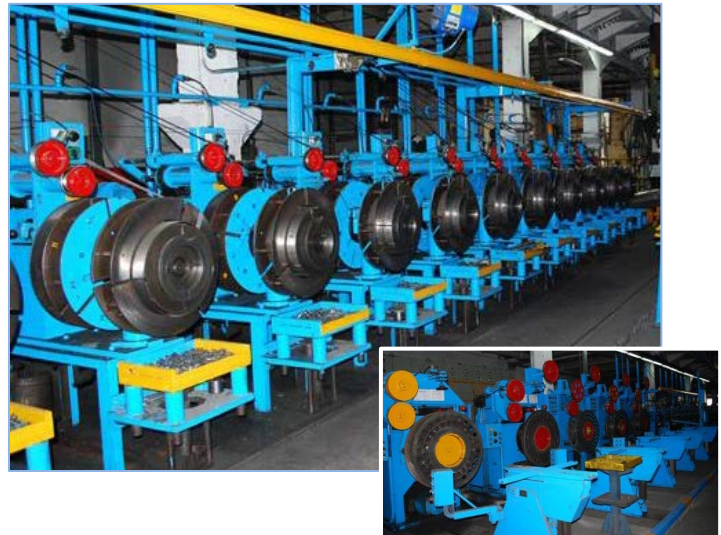
325MM x 1.27MM-0.5MM 5TON OSCILLATING STEEL STRAPPING LINE, 12.7mm-32mm, 16 OSCILLATING RECOILERS
