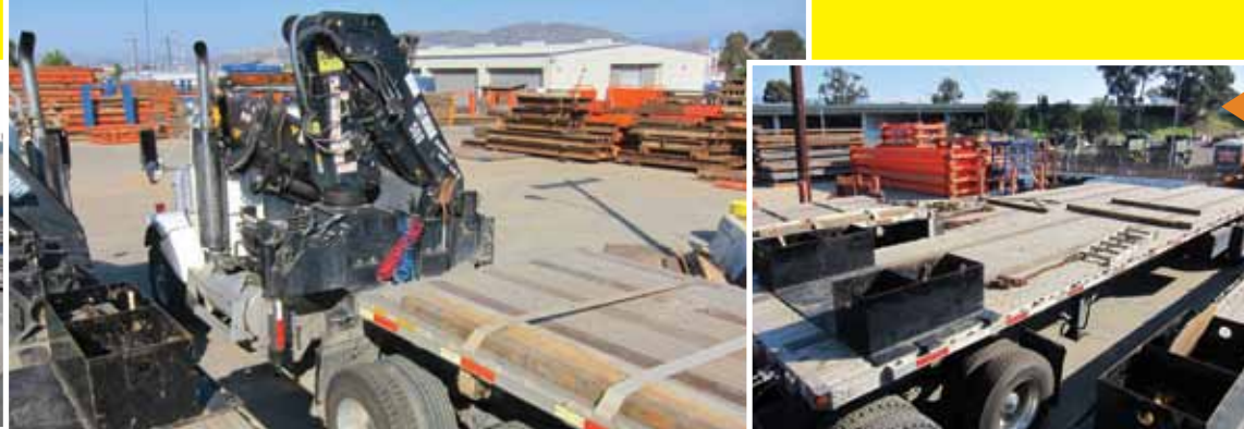
2004 Freightliner Truck Tractor with Hiab 500 boom and utility flatbed
