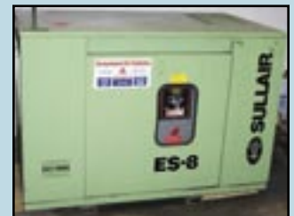
SULLAIR 62 HP. ROTARY SCREW AIR COMPRESSOR
