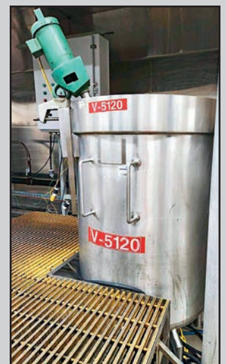
JACKETED MIX TANK
