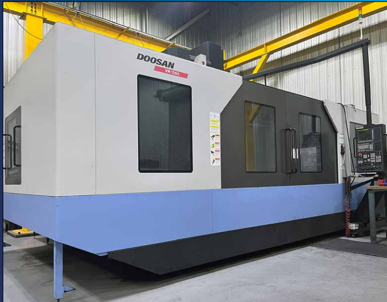
2014 Doosan M1260 CNC Vertical Machining Center
