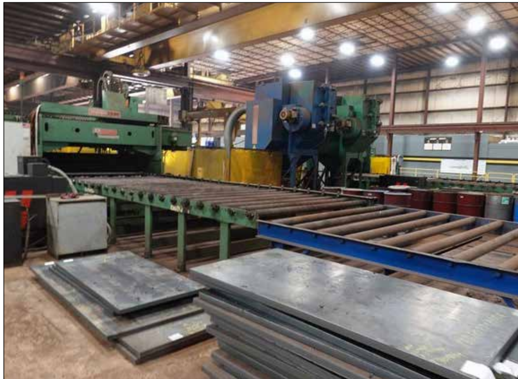
Peddinghaus Model HSFDB-2500/B Plate Processor
