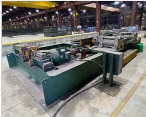
Bay Lynx BC 1200 Beam Cambering Machine
