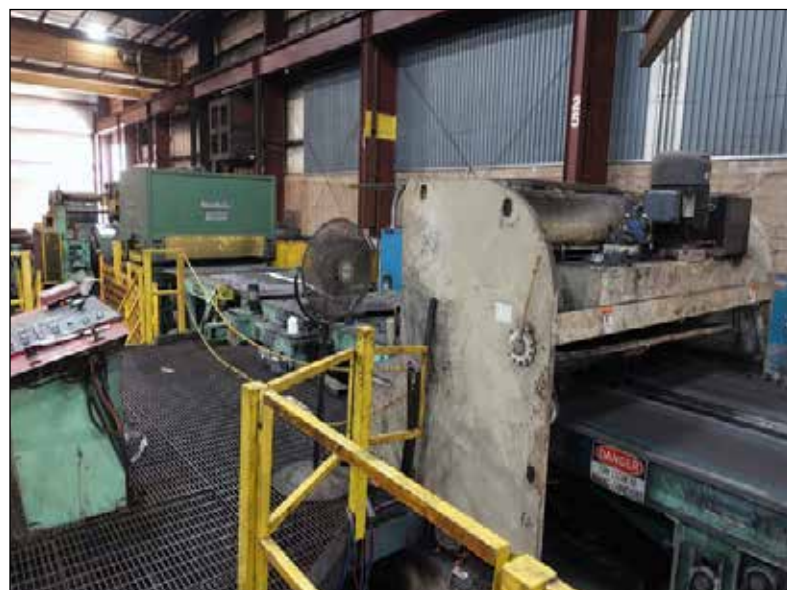
72" x 1/2" x 44,000-LB Cap Cut-to-Length Line
