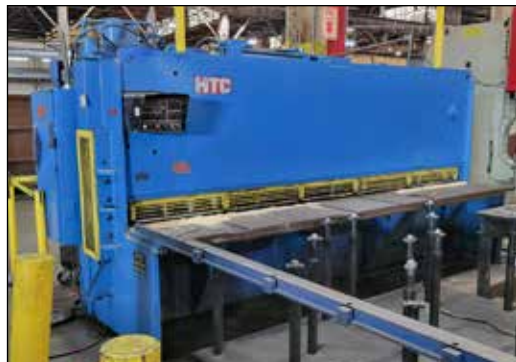
HTC 12' x 3/8" Hydraulic Power Squaring Shear
