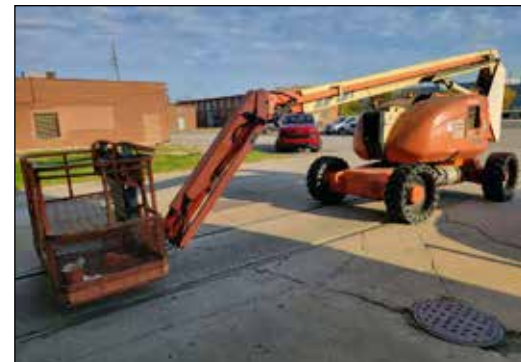
JLG 600AJ, 60' Articulating Boom Lift
