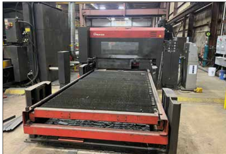
Amada Laser Model FOM2-RI-3015, 4000 Watt
