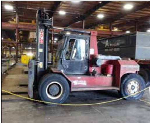
Taylor Forklift Model TE 300M, 30,000 LB Cap
