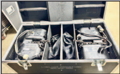
1-TON ELECTRIC CHAIN MOTOR HOISTS IN ROAD CASE
