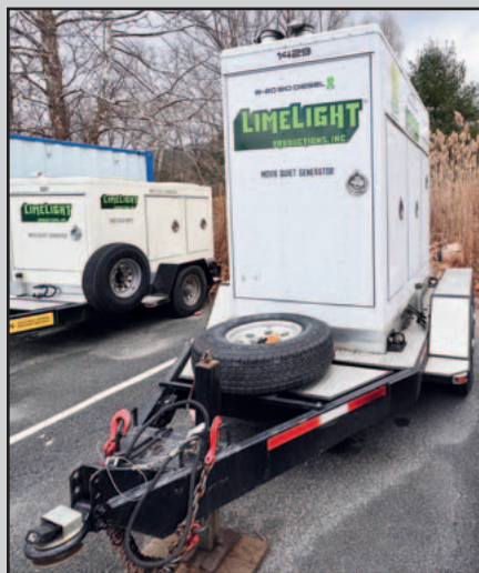
(1 OF 3) MQ POWER 1400 AMP MOVIE QUIET DIESEL TOW PLANTS
