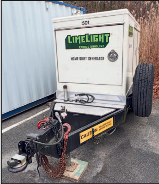
MQ MOVIE QUIET 500 AMP DIESEL GENERATOR
