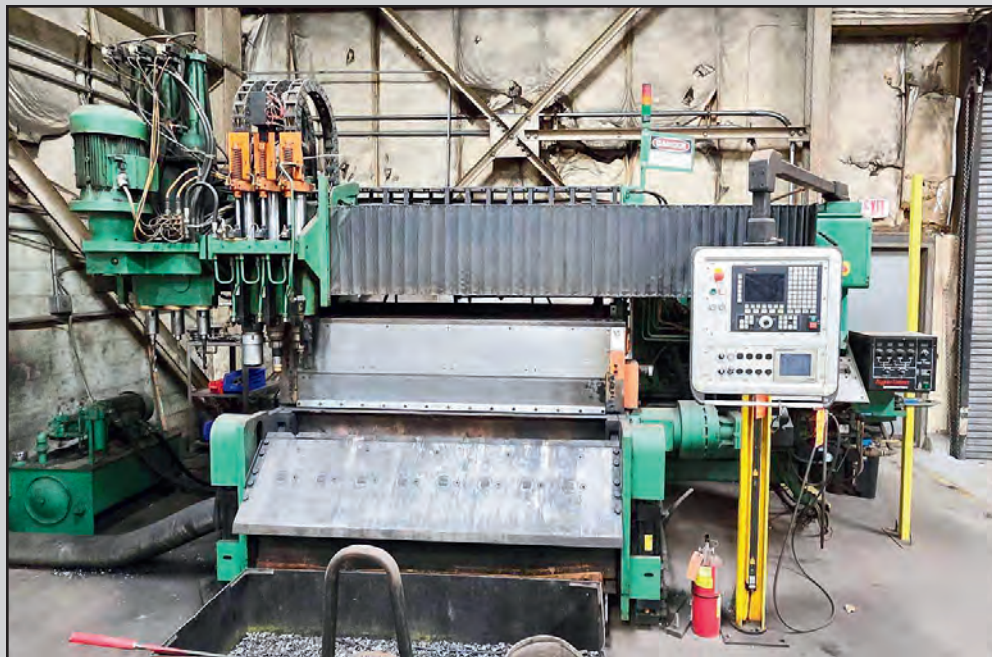
REBUILT PEDDINGHAUS CNC PLATE PROCESSING LINE
