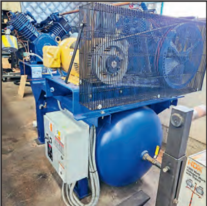
15 HP QUINCY COMPRESSOR
