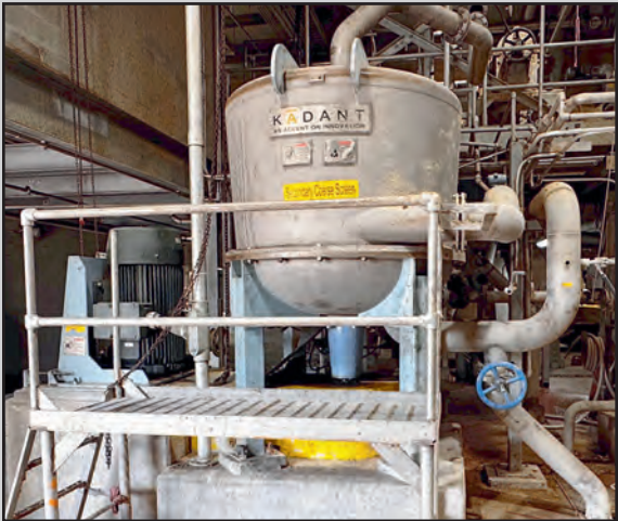
KADANT STAINLESS STEEL PRESSURE SCREEN
