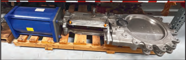
STAINLESS STEEL 18" KNIFE VALVE WITH ACTUATOR
