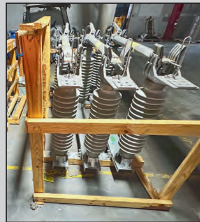
2024 SOUTHERN STATES 72.5 KVA VERTICAL BREAK DISCONNECT SWITCH
