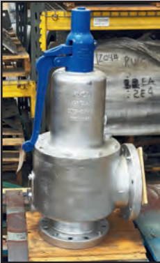
KVC 12" STAINLESS STEEL PRESSURE RELIEF VALVE
