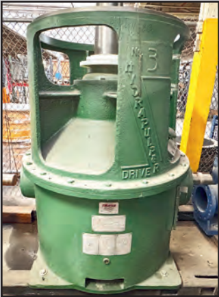
(1 OF 2) REBUILT BLACK CLAWSON NO. 3 HYDRAPULPER DRIVES
