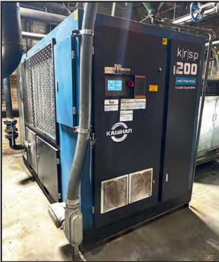
KAISHAN 200 HP ROTARY SCREW AIR COMPRESSOR
