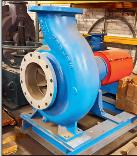
REBUILT 316 SS GOULDS CENTRIFUGAL PUMP
