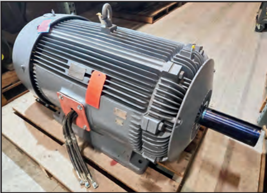
REBUILT 200 HP MOTOR
