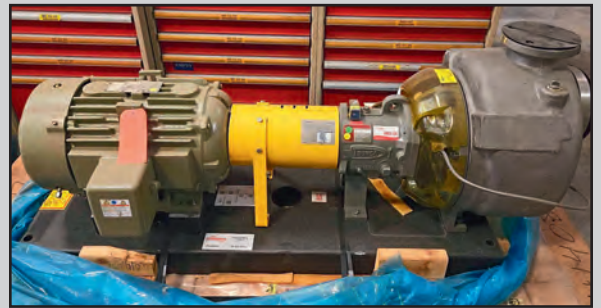
4 X 3 FLOWSERVE PUMP SKID
