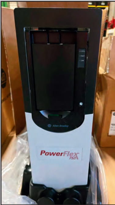
ALLEN BRADLEY POWER FLEX AC VARIABLE SPEED DRIVE CONTROL
