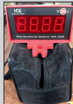
HIGH VOLTAGE AC AMMETER
