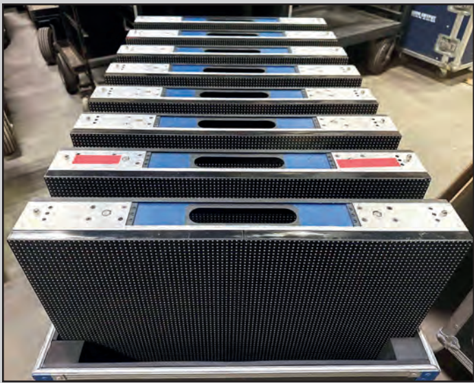
(8 OF 88) ELATION EPT-16P VIDEO WALL PANELS IN ROLLING CASES
