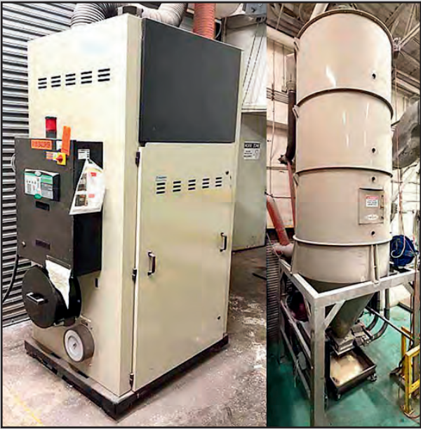
CONAIR DRYER SYSTEM
