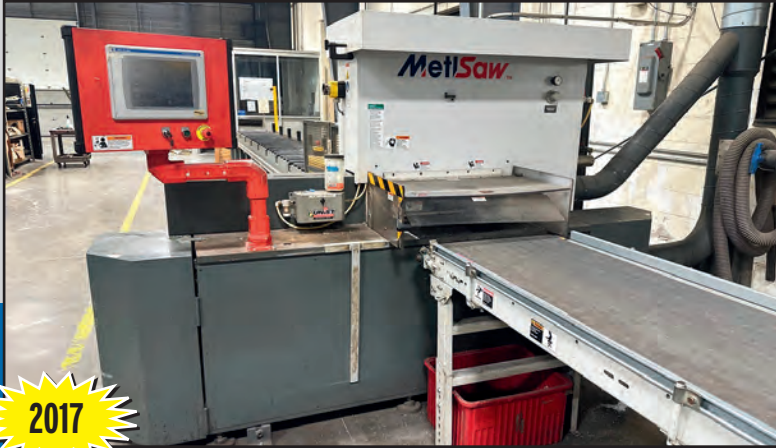
METLSAW CNC COLD SAW WITH CABLES
